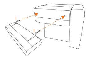
From the underside of the seat base via the zippered compartment, attach the flat washer **(H)**, spring washer **(G)** and the hexagon nut **(F)** to the headrest stem and fix firmly using the socket wrench. Close the zipper compartment and return the sofa to an upright position.
