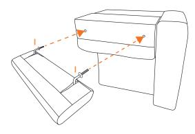
From the underside of the seat base via the zippered compartment, attach the flat washer **(H)**, spring washer **(G)** and the hexagon nut **(F)** to the headrest stem and fix firmly using the socket wrench. Close the zipper compartment and return the sofa to an upright position.
